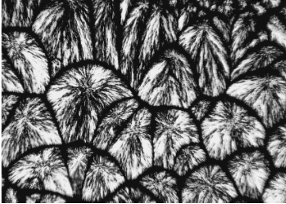
Figure 5 Typical 50/50 directionally solidified sample with atactic interfaces (Sample 22, 1050 \times 1600 \mu\text{m} ).
