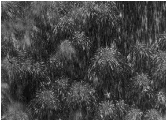
Figure 7 Unidirectional \alpha -phase crystalline structure often present in early stages of directional solidification (Sample 27, 1050 \times 1600 \mu\text{m} ).
